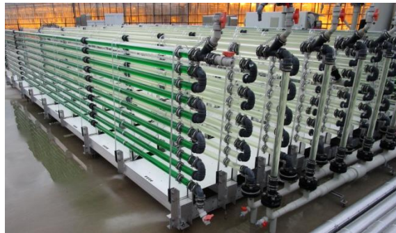
Figures 2 and 3. GWP®-III reactors at F&M pilot plant (Florence-Italy) and horizontal tubular for outdoor microalgae cultivations at AlgaePARC (The Netherlands)
